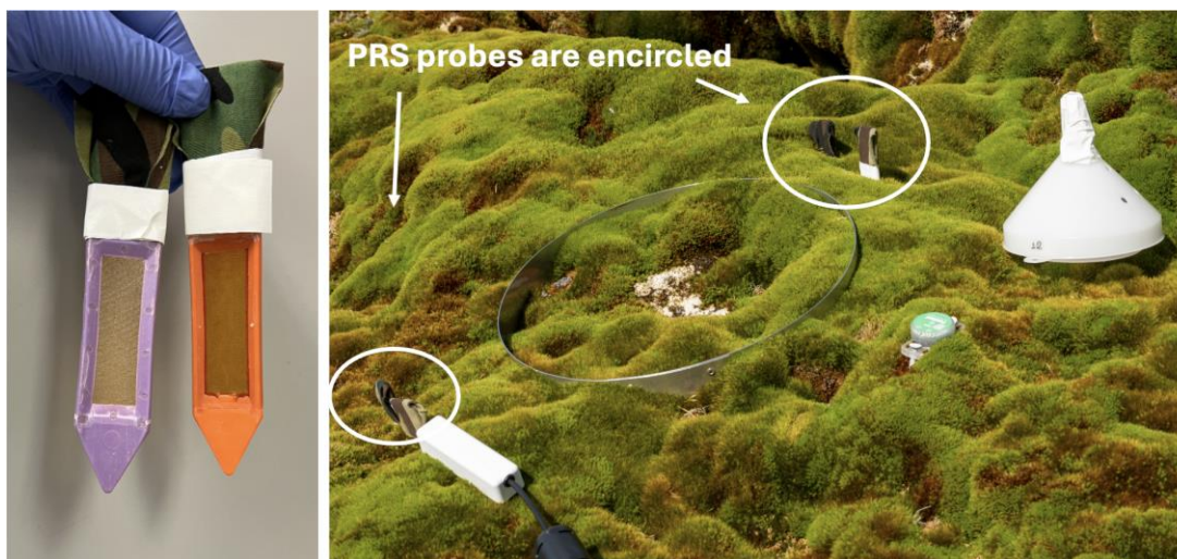
Figure 3- Plant Root Simulator probes (PRS® probes, Western Ag Innovations) are used to quantify soil fertility. These “sticks” provide minimal disturbance, while giving valuable information on soil nutrient availability over a longer time period. The sticks are covered with strips from a camouflage shirt to (try to) outsmart curious skuas at our sites. Image credit: Natasja van Gestel
